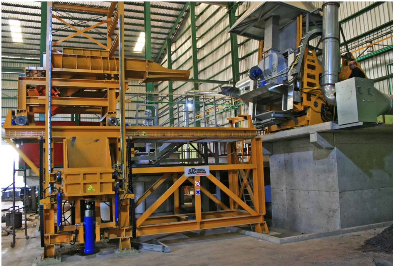
Fig 19: Automated furnace charger and furnace (Courtesy of Green Recycling Industries Ltd., Agbara, Nigeria, and STC, Italy).
