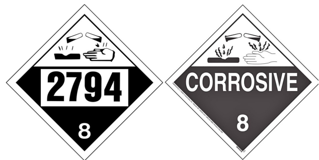
Figure 8. Two typical UN 2794 HAZMAT Class 8 decals commonly seen on vehicles transporting WLABs.
