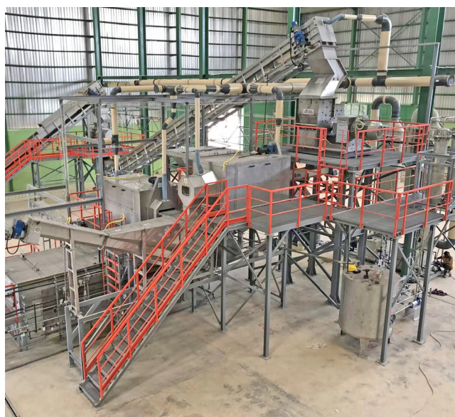
Figure 14: WLAB automated hammer mill breaker. (Courtesy of Green Recycling Industries Ltd., Agbara, Nigeria, and STC, Italy)
