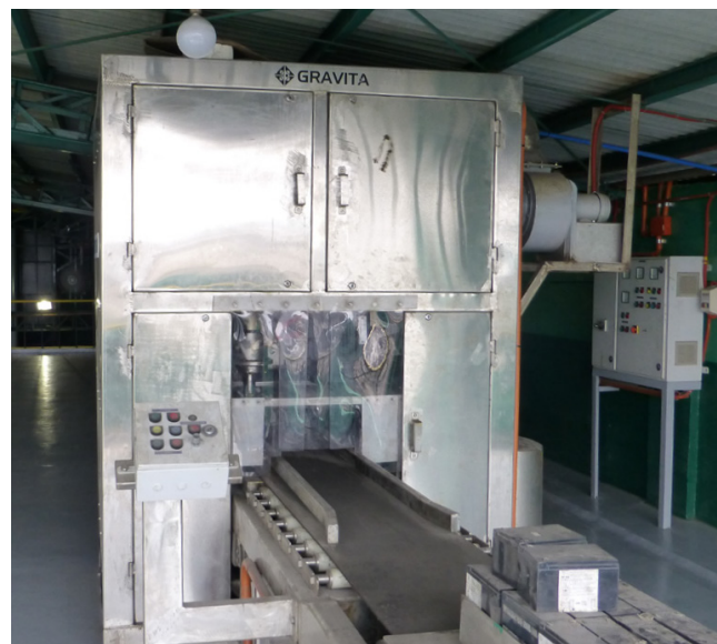
Figure 13: Ventilating battery saw. (Courtesy of Gravita, India)
