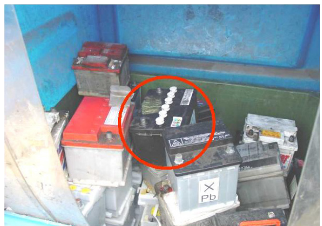
Pic. – A ULAB with the terminals and caps proud of the top of the battery (Red Circle). Fortunately, this ULAB was on the top of this pile in a London collection skip.
