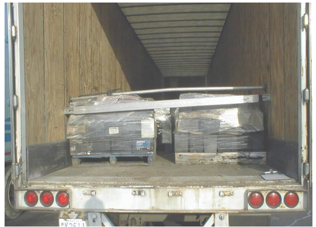
Pic. – Properly blocked back row to prevent movement of the palletized ULAB
