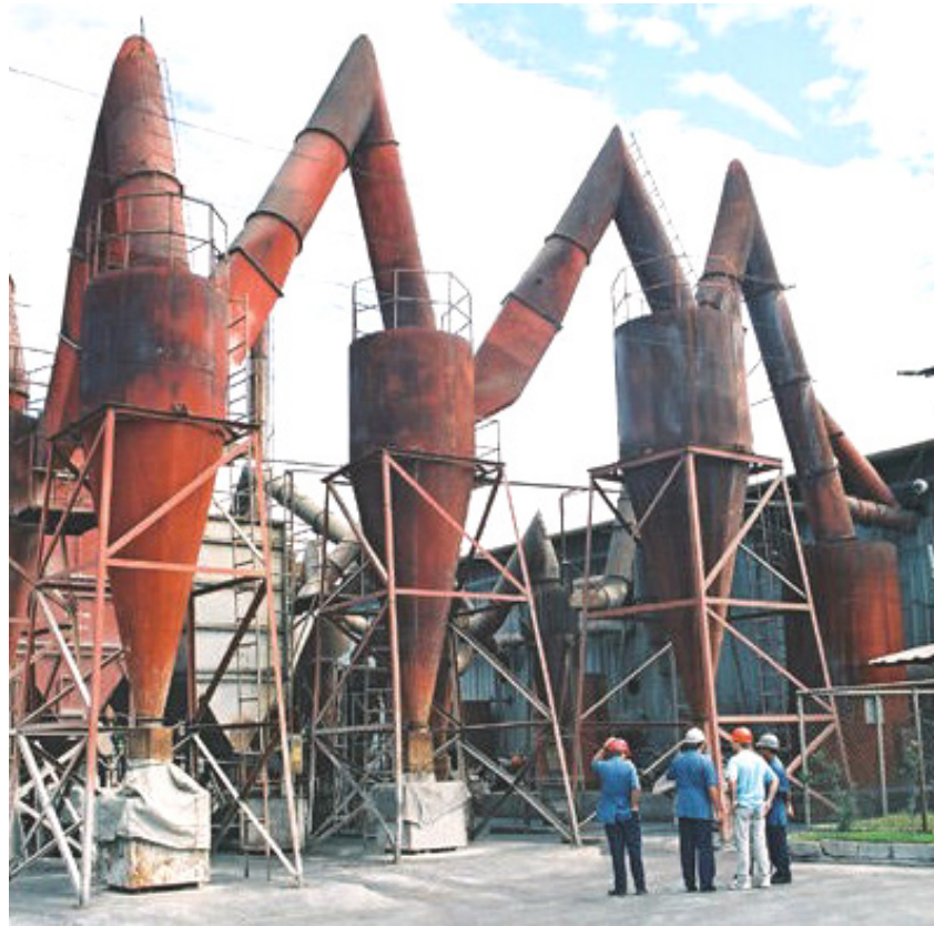
Pic. Cyclones in series at the Baterias de El Salvador plant in San Salvador
