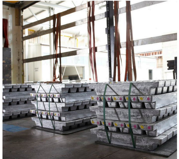
At the end of the recycling process lead ingots are ready to be reused in a variety of applications
